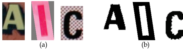
Fig. 6. Examples of binarization using a maximum separability axis in a color space. (a) Input images. (b) Binarized images.
