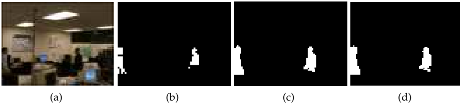
Fig. 8. Low contrast videos: (a) Handshake video sequence. Detected foreground regions using (b) AKDE. (c) RM. (d) SVDDM.
