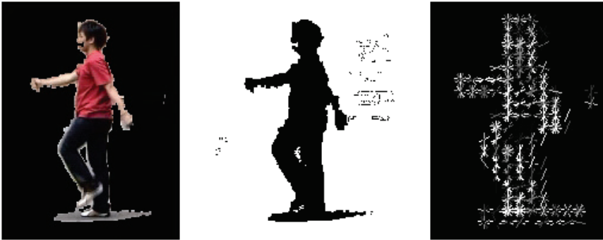
Fig. 9. Images walking leftward. The left image is the input image, the middle image is the silhouette image, and the right image is the HOG features image.
