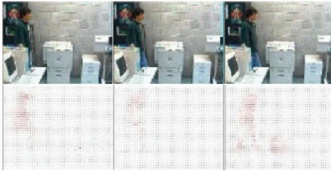
Fig. 2. Example of OF, in red the vectors of the flow of the moving person
